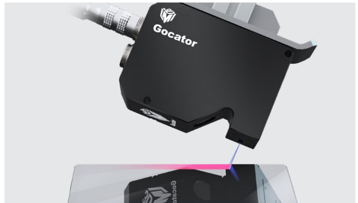
Gocator® 2512 scanning cell phone cover glass assembly
