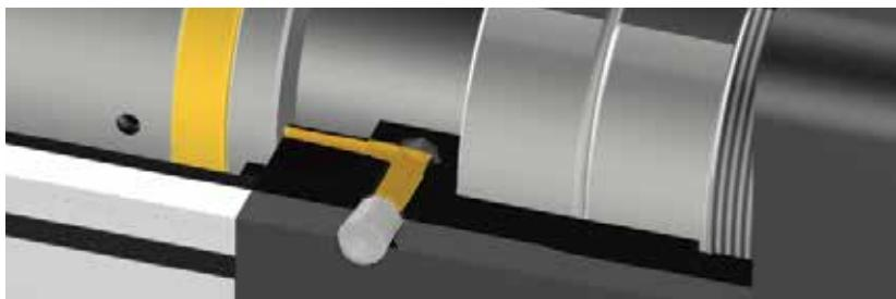
Relubrication is simple with the easy access port. Users simply perform a controlled retract of the cylinder approaching the endstop under slow speed and grease the cylinder.
