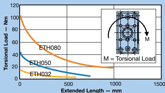
\* Deflection curves represent cylinders mounted in any orientation
