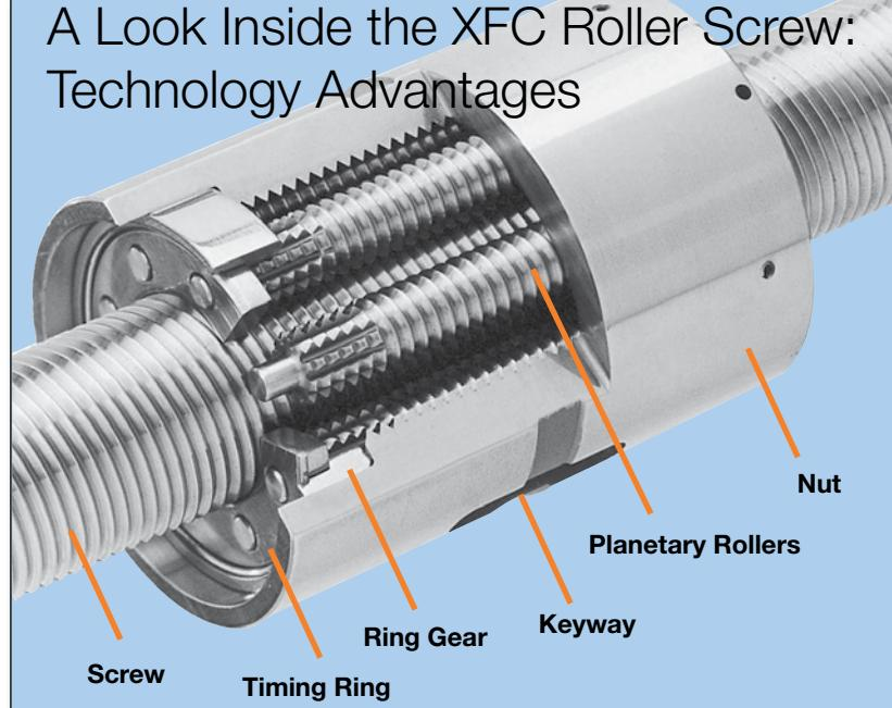
Planetary roller screws offer distinct benefits over traditional ball screw and lead screw mechanisms, and add features not easily attainable with hydraulic or pneumatic linear devices.
