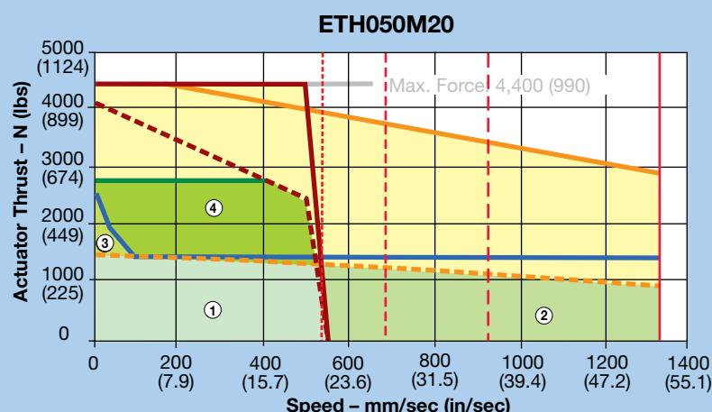
\* Maximum thrust assumes a cylinder mounting orientation with a fixed mounting position and a guided load. For limitations on column buckling, please see page 43.
