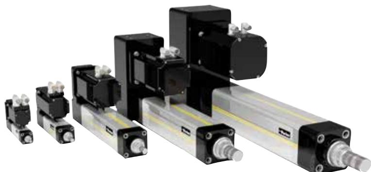
ETH cylinders are available in five sizes with 32 up to 125 mm profiles. Both in-line and parallel motor configurations provide stroke lengths up to 2000 mm and speeds to 1.7 m/sec.
