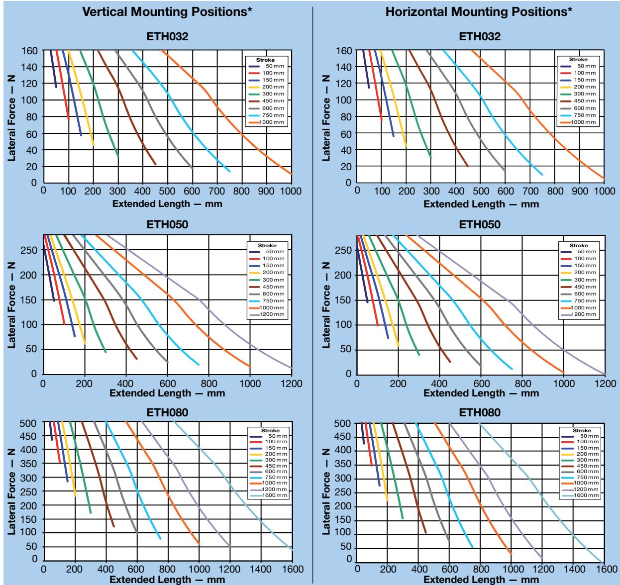
\* The diagrams apply for a medium travel speed of 0.5 m/s, an ambient temperature of 20°C and all housing orientations.
