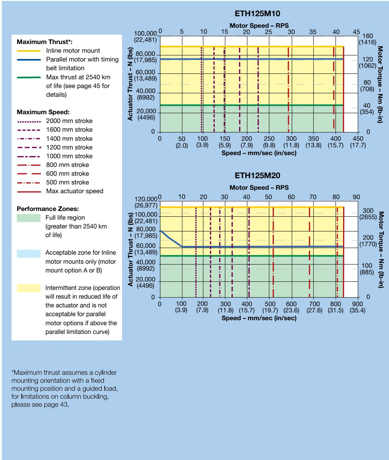
\*Maximum thrust assumes a cylinder mounting orientation with a fixed mounting position and a guided load, for limitations on column buckling, please see page 43.
