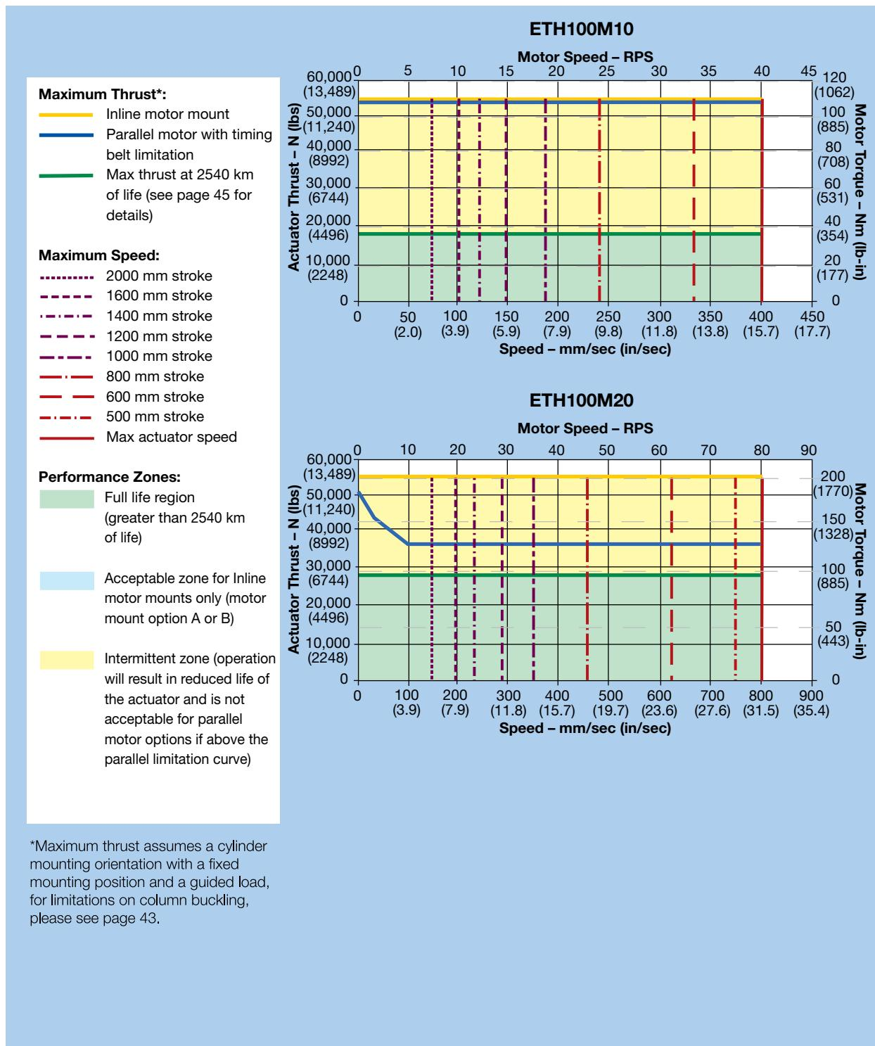
\*Maximum thrust assumes a cylinder mounting orientation with a fixed mounting position and a guided load, for limitations on column buckling, please see page 43.
