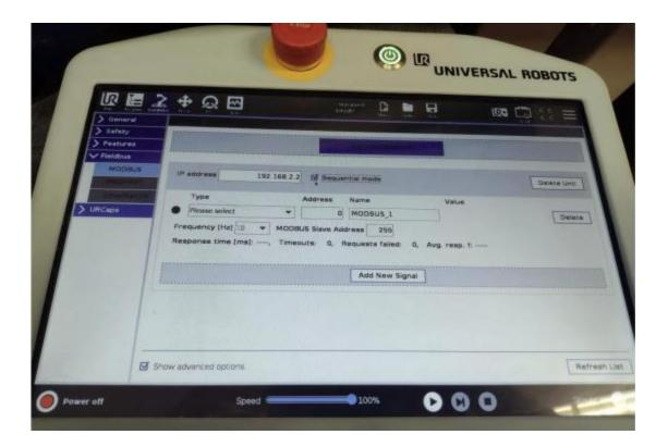
16. After this is set-up, you'll be able to add the signals that the 3S80/EV7 system has been configured to read, in our case, the X and Y positions. For this example, we would set-up two signals, one with the Address configured for the X Position, and the other with the Address configured for the Y Position. For clarity, you can rename the signals to what makes most sense to you.
