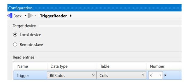
8. The trigger step can be set up in multiple ways. In this case, a loop was implemented. The flowchart does not execute unless a trigger is received via ModbusReader, which serves as the break condition for the loop.
