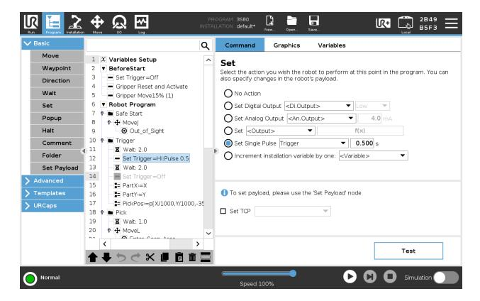
The screenshot above shows how to integrate a "Trigger" function, where the robot will send a pulse via MODBUS to the 3S80, which in turn will trigger the camera to take a new picture/capture. This is not necessary, but allows for the system to become fully autonomous, not requiring the user to take a new snapshot after every pick and place.
