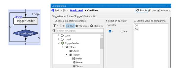
9. To finalize the vision parameters section, a trigger step was implemented to control the image acquisition of the 3S80.
