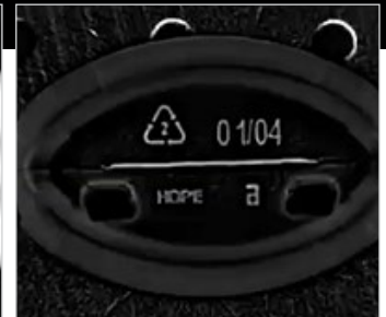
With SurfaceFX: Noise is removed and embossed features are visible.
